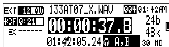
reversed numbers indicating that recording is active
